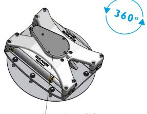
Fin actuator assembly may be installed in any convenient radial 360° position in the hull.
